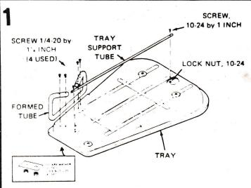
Place cart tray upside down on convenient work surface. Attach both ends of tray support tube to tray with 10-24 by 1-inch truss head screws and Lock nuts.
