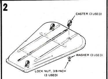
Place shafts of all casters through holes as shown. Turn tray over and attach casters securely to tray with washers under the 3/8-inch Lock nuts.
