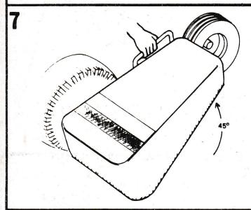
To empty the basket, lift the formed tube out of the deck bracket. Remove the entire catcher assembly, open the zippered end of the basket, and dump out clippings.
