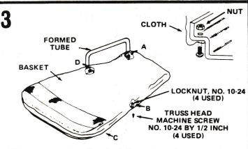
With support wires flat (and three loops in wires pointing downward) place Basket on tray so notched opening of basket is aligned with notch in edge of tray. Slip front end of basket under lip of tray and secure grommet at A to tray with one No. 10-24 by 1/2 inch Truss Head Machine Screw and one No. 10-24 Locknut.
