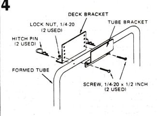
Attach tube bracket to deck bracket in bottom hole with two 1/4-20 by 1/2-inch truss head screws and 1/4-20 Lock nuts. Do not tighten nuts.
