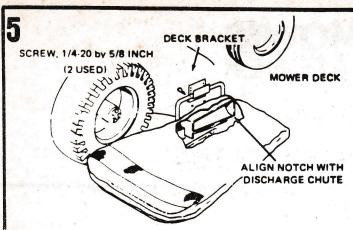
Place assembled tray, basket, and deck bracket against side of mower so front edge of notch in tray is aligned with front of mower discharge chute. Set deck bracket on mower deck and scribe marks on deck for two holes required to mount bracket. Center-punch marks and drill two 1/4-inch holes through deck.
