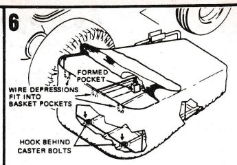
Unzip end of basket. Pull rear support wire back and hook behind attaching bolts on casters. Make sure depressed parts of top wire slide into pockets provided in cloth basket. Raise front of basket by pivoting side support wires down and hooking between sides of tray and formed pocket and bolts. Close zipper.
